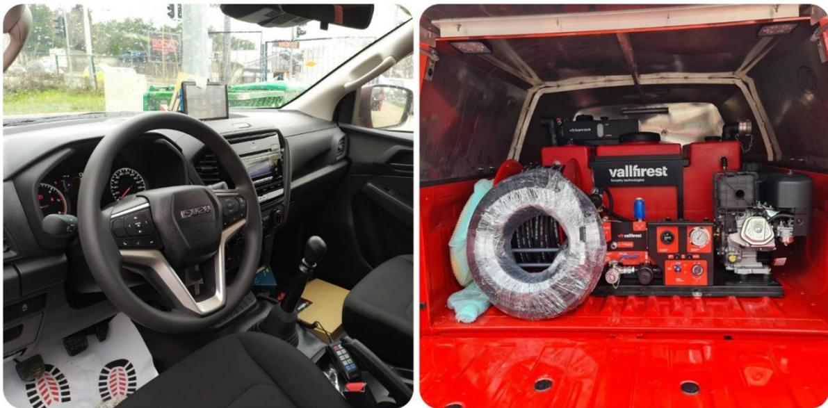
Picture 2 - Delivery of firefighting vehicles with UHPS pumps – cabin and UHPS compartment
